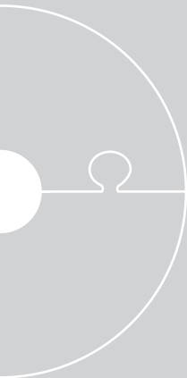
click-one-two® Ø 55 mm PEX-Rohr = 12 mm Loch
