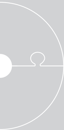
click-one-two® Ø 55 mm PEX-Rohr = 10 mm Loch
